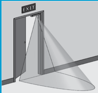
Motion sensor shown adjusted for door approach
